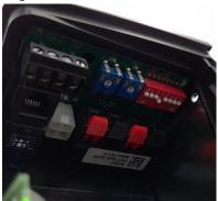
It is only possible to set DIP switch 1 if the operator is not 'taught in'. If you change the DIP switch on a taught-in operator, an error (flashing 8 ×) will display when trying to operate the door.
