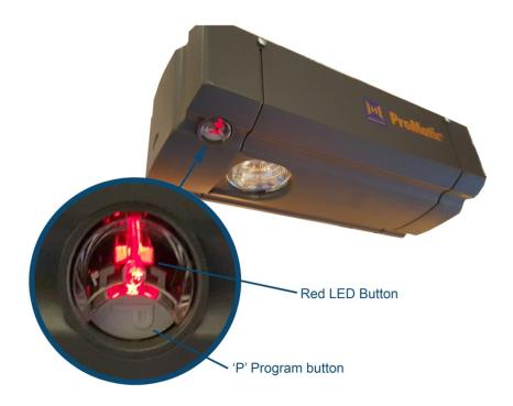
Please make sure the door is set to operate automatically before resetting (see Manual and Automatic operation info sheet)
