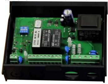
Connections 5 and 8 from each relay output would normally provide the open and closed relay switching connection to the automation systems.
