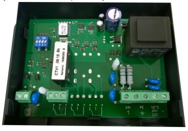
Connections 5 and 8 from the relay output would normally provide the open and closed relay switching connection to the automation system.
