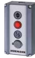
Push button DTH-IM To move the door into the Open / Close positions, separate stop button to stop door travel, 1/2 Open button to open the door up to the programmed intermediate travel limit, with miniature lock: operator control is deactivated, operator movement is no longer possible (2 keys included in the scope of delivery)
