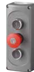
Push button DTN A 30 For separate control of both operational directions; stop button is a push-to-lock button which, once pressed, stays depressed in order to prevent unauthorised operation; subsequent actuation is then only possible through unlocking with a key (2 keys included in the scope of delivery)
