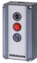
Push button DTH-I To move the door into the Open / Close positions, separate stop button to stop door travel, 1/2 Open button to open the door up to the programmed intermediate travel limit, protection category: IP 65,
