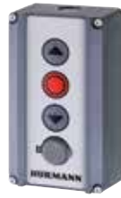
Push button DTH-RM Separate control of both operational directions; separate stop button, with miniature lock: Control of the operator is deactivated – operator movement is no longer possible (2 keys included in the scope of delivery)
